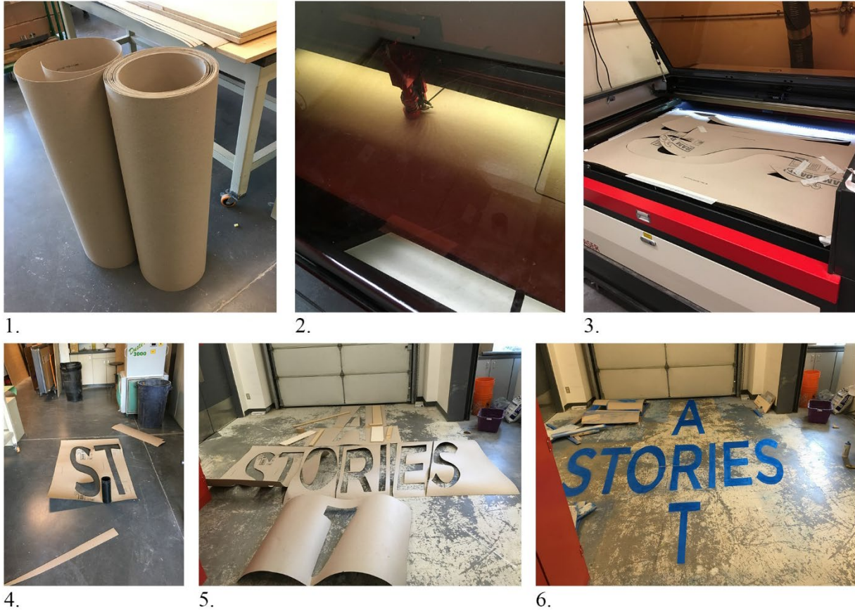
Figure 9. Kits-of-Parts fabrication process: 1. Cardboard (Ramboard) cutting medium. 2. Laser cutting Ramboard. 3. Complete laser-cut component. 4. Component assembly. 5. Complete component assembly (kit-of-parts). 6. Spray chalk paint application.
