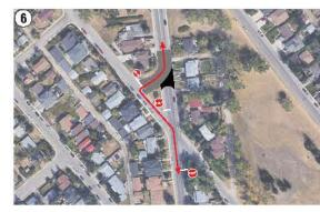
The traffic diverter concept can be applied to the intersection of 48 Street and 23 Avenue by creating deviation of 48 Street from a straight line roadway to a minor roadway with stop control. With added stop control of three seconds, traffic will come to a stop with significant reduction of travel speed and a
