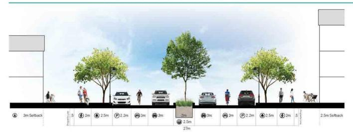
Option A: One Direction Cycle Track with Median Stormwater Tree Planters
