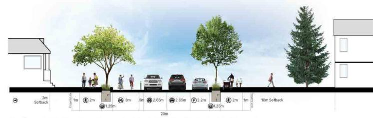
Option D: Bi-Direction, Separated Cycle Track with Curbside Bioswales
