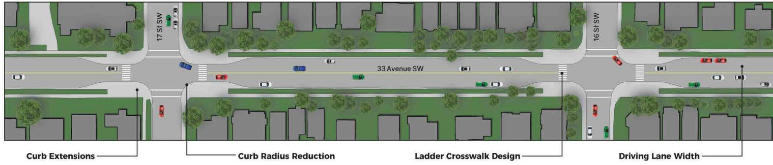
Curb extensions make intersections safer for pedestrians by making them more visible to vehicles. reducing the crossing distance and eliminate driving in the parking lane.
