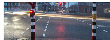
Lower position of lights can be seen by drivers when sun is in eyes Podegaren, Netherlands
