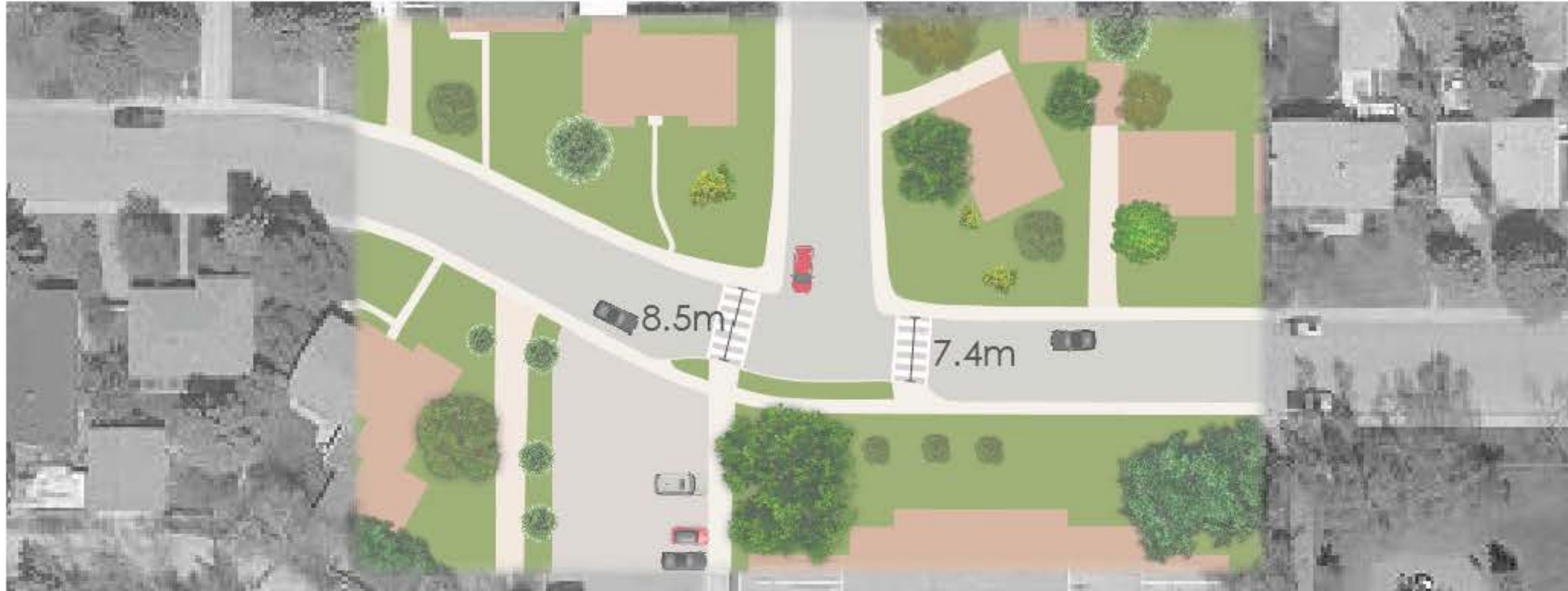
Dimensions of the proposed intersection at 87th Ave and 11th St.
