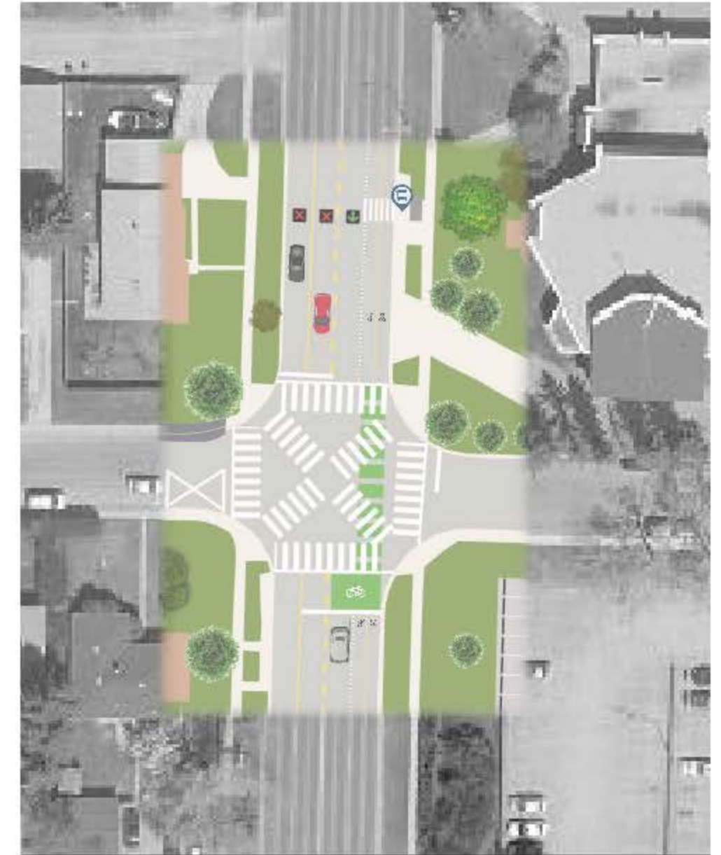
An illustration of the proposed lane and crosswalk changes at Elbow Drive and 89th Ave SW.
